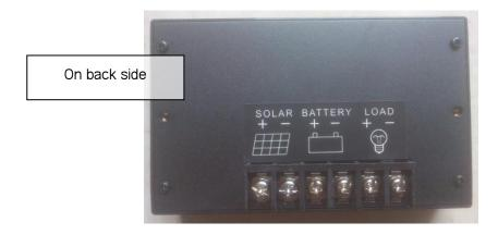
3. Then turn on Switch/breaker to start charging the battery
